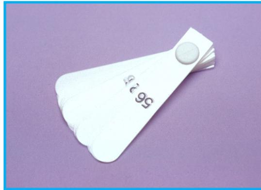
A leaf gauge is a very simple device similar to a “feeler gauge” except all leaves are of the same dimension of almost exactly 0.1mm thick. This gives the operator a very easy recording of the exact number of leaves measuring the exact amount of opening in mm’s (eg. 5 leaves equals 0.5mm opening; 17 leaves equals 1.7mm opening).
