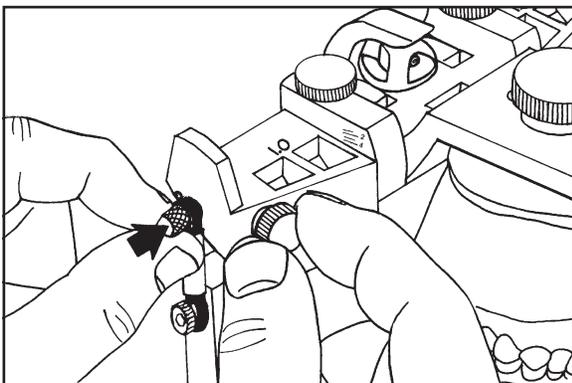
Reinsert right and left Dyna-Link pins (arrow) and lock in place with retaining thumb screws. Release elastic centric latch hold down and engage centric latch over centric pin cap.
