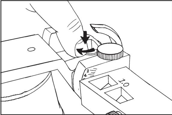
then depress centric pin cap and rotate clockwise (arrows).
