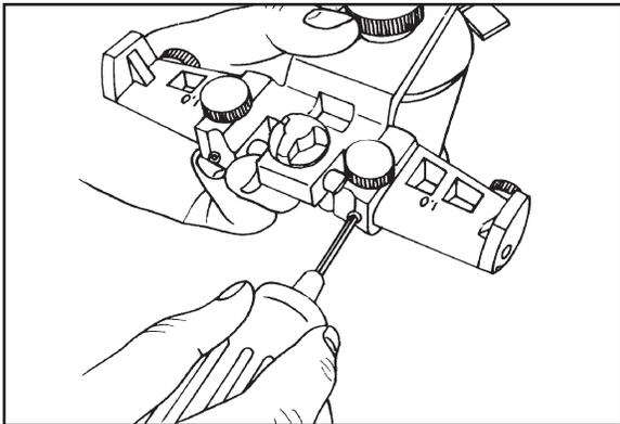
After analog angulations have been obtained, make sure analogs are in contact with calibrated sides of articulator. Tighten both analog axis shaft lock screws with hex wrench to retain analog angulation.
