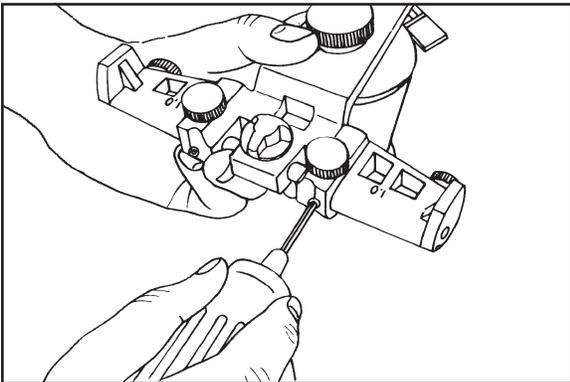
Loosen right and left analog shaft lock screws with hex wrench.
