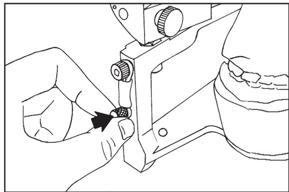
Release centric latch (arrow) to allow centric pin to spring upward and lift lower end of pin out of centric channel in mandibular frame. (If centric pin does not spring upward when latch is retracted, rotate centric pin cap to release it.)
