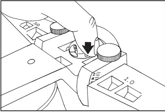
To lock centric locator pin in down position when centric latch is disengaged, place finger on flange of pin cap (arrow)
