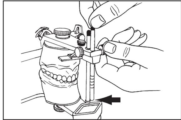
Loosen thumb screws and retract right and left Dyna-Link pins (arrow).
