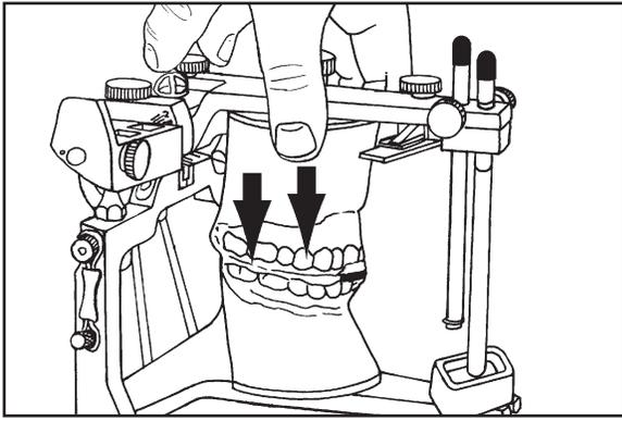
While maintaining downward pressure on casts (large arrow), loosen left side axis shaft thumb screw to obtain angular inclination for left side. If analog does not rotate freely downward into contact with condylar element, tap lightly on upper anterior surface of analog.
