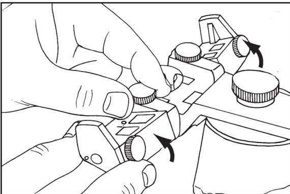
Rotate and lock both motion analogs in their "0" positions using only thumb screws to maintain position. The "0" line should be equal to the upper surface of the analogs. The analogs should be in contact with the calibrated sides of the articulator.
