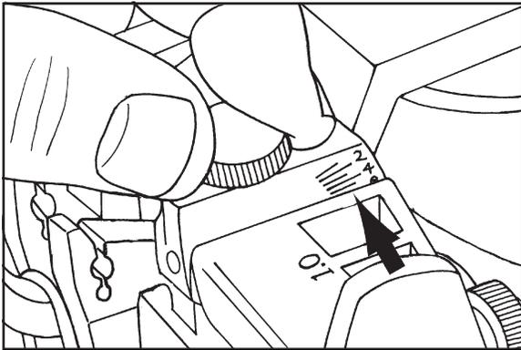
Angular setting is read where upper surface of analog corresponds to a calibration line on side of articulator (arrow).
