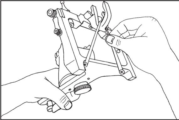
Stretch elastic band on lower surface of mandibular frame over extending latch arm to keep latch retracted back and down out of the way.
