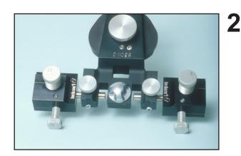
The large screw on the top of the housing can be adjusted to move axis element on the articulator up and down. The large screw on the back of the housing can be adjusted to move axis element on the articulator forward and back. The small thin screws are just lock screws for the larger adjustment screws.
