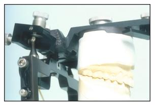
When both large screws are flush or equal to the inside surfaces of the housing and the lines on the head of the large adjustment screws are equal to the line on the housing, that is the centric position. One full turn of each screw is equal to 1mm.
