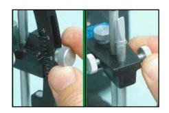
2. Set Adjustable Platform to the zero position with the adjustment screw.
